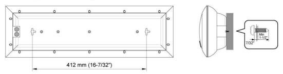
Fasten screws into a firm wall or wall support as shown in the figure, and hang the holes of the mounting bracket on the protruding screws.
